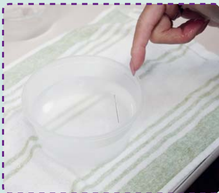
Floating needle — to learn how water surface tension will keep a needle lying on the surface of water
